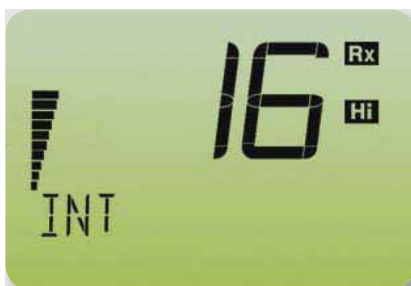
When turned on, channel 16 will automatically be selected.
